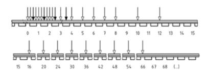
SLR utilised LMS SCADAS data acquisition equipment and Test.Xpress analysis software to record the time domain force and acceleration data, as well as calculate accelerances and coherence for review on site. The sampling frequency was 20.48 kHz. 10 impacts (excluding any double-hits) were identified from the peaks in the hammer trace. These peaks and the associated decay were then extracted for analysis following the method described in the standard.
