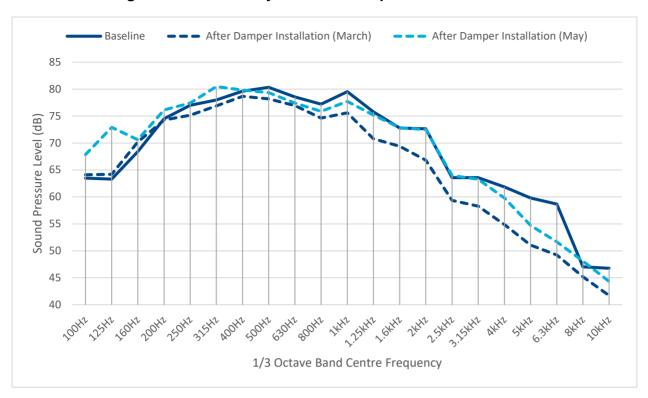
Figure 10 Train Passby Sound Level Spectrums – Location 1
